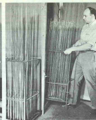
Oven heat is used to "set" the cement. After cleaning, the sections are impregnated with another Bakelite resin and again oven-cured, to become completely Permanized and ready for assembly.
