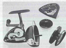
Reel is easily taken apart for inspection. Note simplicity of design and few moving parts.
