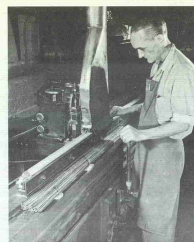
The specially designed milling machine weighs 2½ tons, yet it mills segments as light as 3/100 of an ounce, to a tolerance of one thousandth of an inch.
